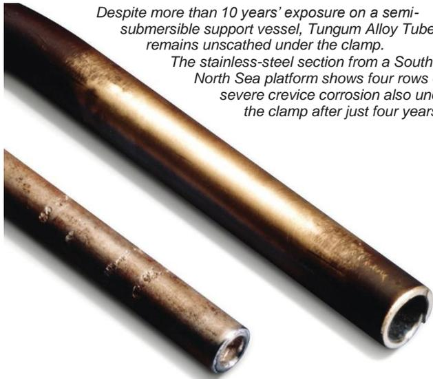
*Despite more than 10 years' exposure on a semi-submersible support vessel, Tungum Alloy Tube remains unscathed under the clamp.
