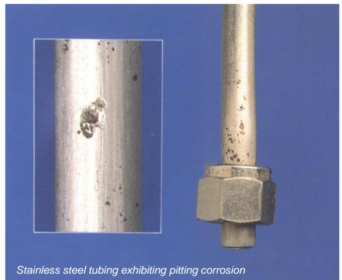
*Stainless steel tubing exhibiting pitting corrosion*
