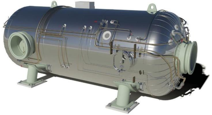
*A Drass hyperbaric chamber showing the gold colored Tungum Alloy Tubing used due to its non-sparking characteristics and excellent corrosion resistance*
