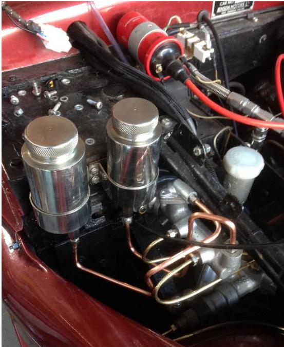
Tony says "As you can see from the brake area photograph, I also polished the 40 year old tubing and then clear coated it as well as the 1/4" copper tubing used on the non- pressure reservoir side. "
