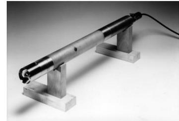
Once at the correct depth, they are expanded by carefully controlled internal pressure so enlarging a cavity in the ground. The cavity size is measured by internal transducers reading to better than one micron. If the instrument is long enough in relation to its diameter, meaning about six times, it turns out that the expansion can be mathematically analysed to give the parameters above.
