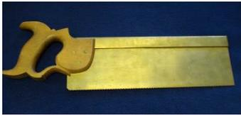
Tungum alloy being a non-magnetic material has always been used on naval minesweepers. As an ancillary item on such vessels tool kits consisting of spanners, saws, scissors etc. were produced for the Royal Navy in wartime Britain.
