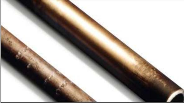
Tungum tube remains unscathed despite more than 10 years marine exposure on a semi-submersible support vessel. The stainless-steel section on the left from a southern North Sea platform, shows both crevice corrosion and chloride pitting after barely 5 years in the same environment.
